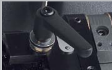
1. 2 side jaws which permits: a) duplication of mortice keys b) duplication of front mortice keys.
