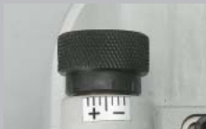
1. Tracer point with micrometric adjustment
